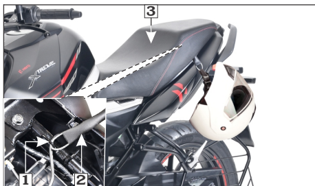
(1) Helmet holder hook (2) Wire helmet set (3) Seat
