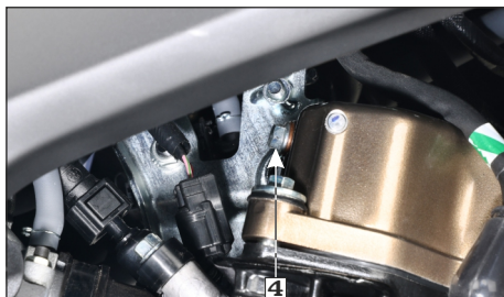
(4) Engine oil check bolt
