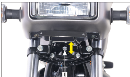
(1) Headlamp adjusting bolt
