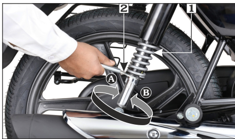
(1) Rear shock absorber (2) Pin spanner (A) Stiffer (B) Softer
