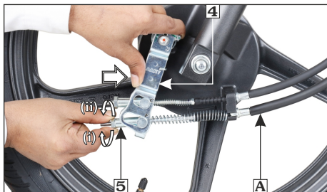
(4) Integrated brake arm (5) First adjuster nut (i) Decrease free play (ii) Increase free play
