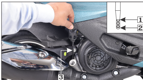
(1) Upper level mark (2) Lower level mark (3) Oil level dipstick
