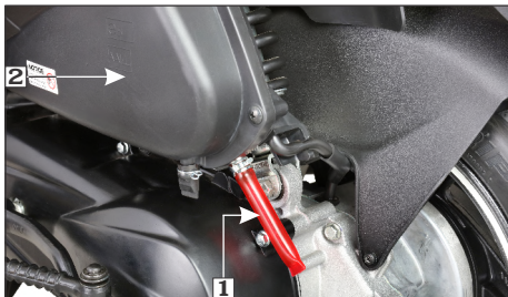
(1) Drain tube (2) Air cleaner assembly
