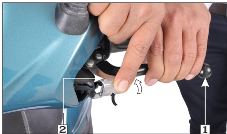
(1) Integrated brake lever (2) Lever lock
