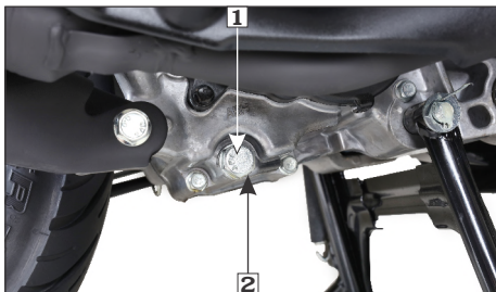
(1) Drain bolt (2) Sealing washer
