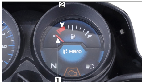
(1) Fuel gauge needle
