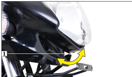
(1) Headlamp adjusting bolt
