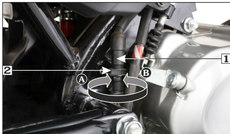
(1) Stop lamp switch (A) Advance
