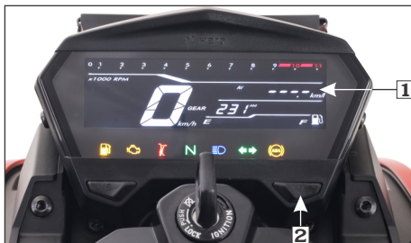
(1) Real Time Mileage Indicator (RTMI) “Av”
