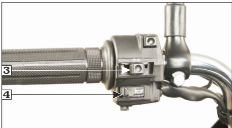
(3) Turn signal lamp switch (4) Horn switch
