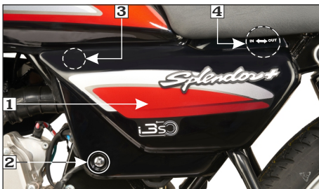
(1) Left side cover (2) Side cover screw (3) Lug (4) Direction indicator
