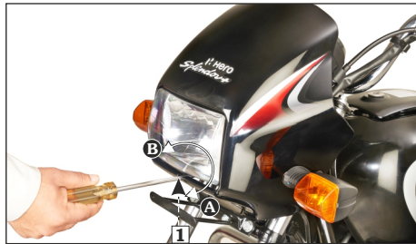
(1) Adjusting screw (A) Clockwise (B) Anticlockwise
