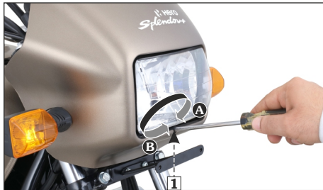
(1) Adjusting screw (A) Clockwise (B) Anticlockwise
