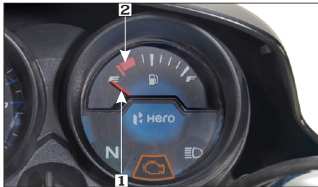
(1) Fuel gauge needle
