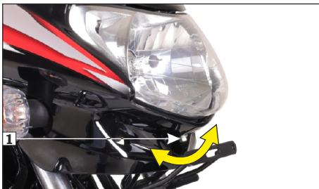
(1) Headlamp adjusting bolt
