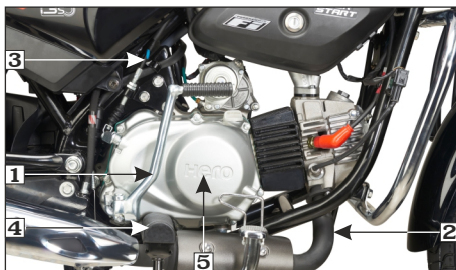
(1) Kick starter pedal (2) Muffler (3) Clutch cable (4) Rider footrest (5) Right crankcase cover
