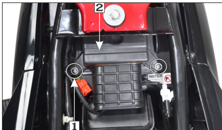
(1) Air cleaner cover screws (2) Cover
