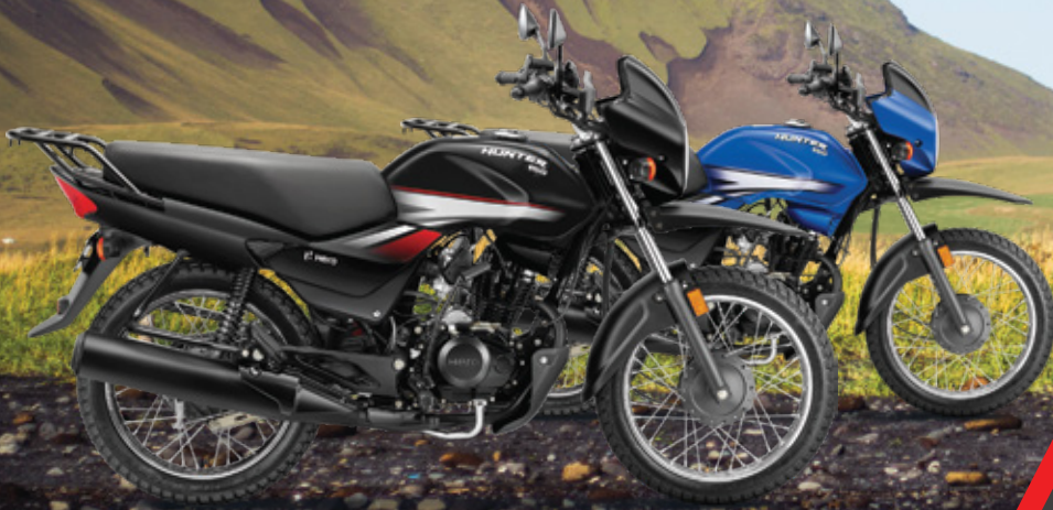
FLAT CARRIER AND SEAT POWERFUL 150CC ENGINE 18" WHEELS WITH KNOBBY TYRES PROTECTIVE BASH PLATE
